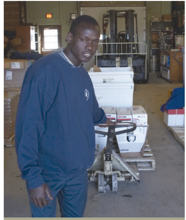
FIGURE 10–2 A pallet jack easily relocates material stored on a pallet and minimizes labor costs.
