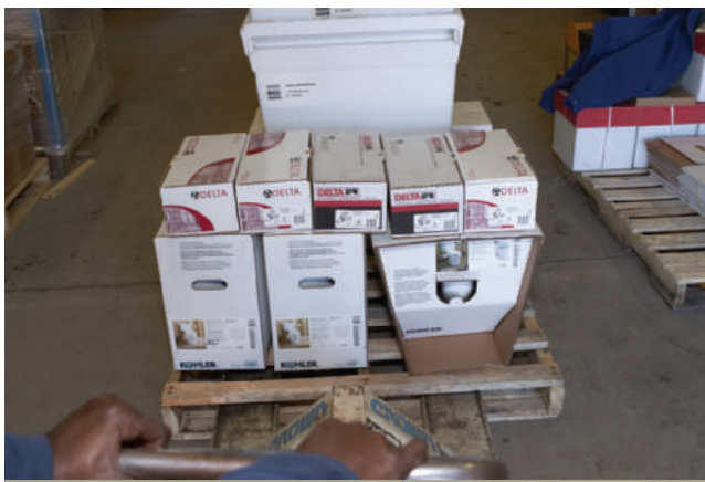
FIGURE 10–1 Organizing material on a pallet to minimize relocating with extensive labor.
