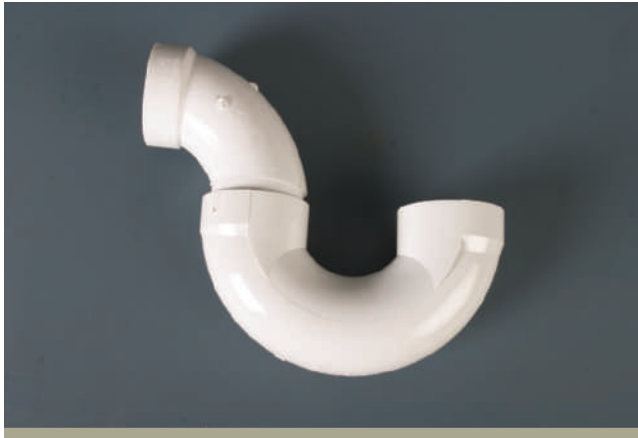
FIGURE 4-34 A p-trap is installed so sewer gas cannot enter an occupied space.
