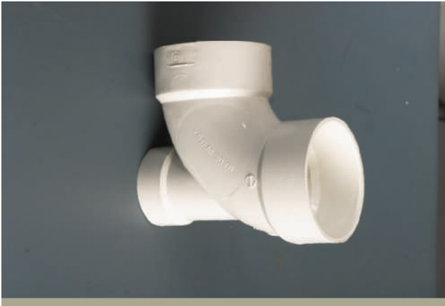
FIGURE 4-32 A heel inlet 90° has specific and limited use in a DWV system.
