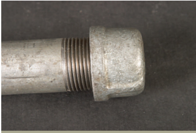
FIGURE 4-21 Galvanized fitting is commonly used to test water distribution systems.
