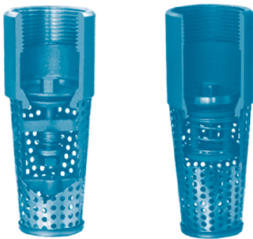
FIGURE 16-16 A foot valve installed at the bottom of the drop pipe serves as a check valve to ensure that the water does not drain back into the well. It has a screen to prevent debris from entering the system.
